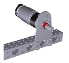
2. Install one NeveRest Orbital 19.2 gearmotor (am-5442) to the Motor Mount plate using three M3-0.5 8mm patched screws (am-1500) in the lower three mounting holes.
