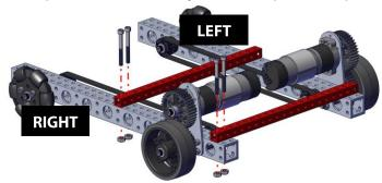
Connect one 12" JST Motor cable to each NeveRest motor at the location shown.
