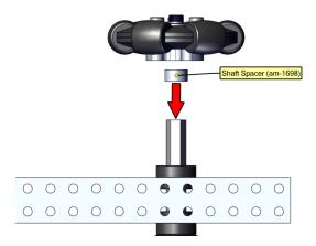
17. Retain wheel with one 10-32 x 0500 inch screw (am-1002) with one #10 washer (am-1026).
