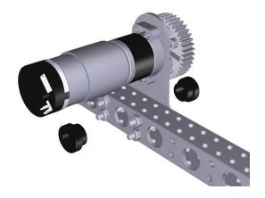
8. Put together two pulley halves (am-4960\_half) to create a pulley.
