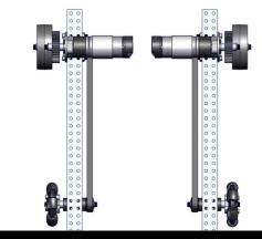
**Note:** Attach the tubes to the center hole pair and the second hole pair on the motor side.
