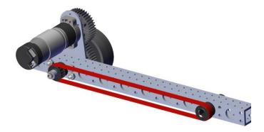
15. Insert the 3 inch shaft assembly through the 14T pulley and previously installed bushings.
