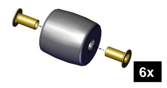
3. Place a roller assembly in between each spoke of the omni wheel half (am-5463\_half).
