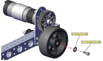
13. Install one 10-32 x 0500 inch screw (am-1002) with one #10 washer (am-1026) into the end of one 3 inch shaft (am-5003-0300).
