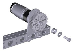
7. Install one  $10-32 \times 0500$  inch screw (am-1002) with one #10 washer (am-1026) into the end of one 4 inch shaft (am-5003-0400).
