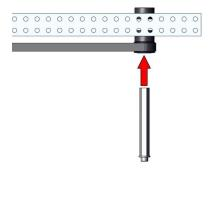
16. Slide one  $\frac{1}{4}$  inch shaft spacer (am-1698) on the shaft from the outside and follow it with one 3 inch omni wheel (am-4967a).
