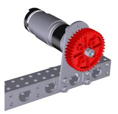
5. Place a  $\frac{1}{4}$  inch shaft spacer (am-1698) on the shaft and retain with one 10-32 x 0500 inch screw (am-1002) with one #10 washer (am-1026).
